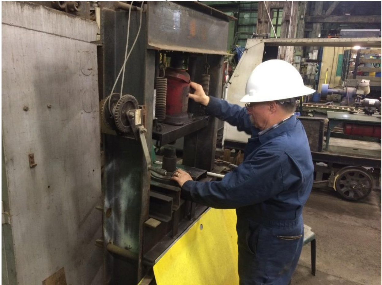
Mike H. using the press to press-out the bearing from the vibrator motor on the work-head of the new-old tamper
